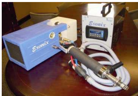
Figure 3-2: UIT device with water cooling and generator
